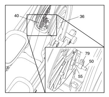
Then, retighten the Screw. Turn one of the crank arms (36) for a moment. Repeat until the console displays correct feedback. When the Reed Switch is correctly adjusted, replace the convenience tray and reattach the left and right side shields.
